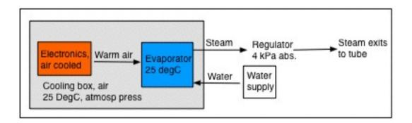
The cooling system will consist of a cool-box maintained at atmospheric pressure, for all the electronic components. The cool-box is chilled by a water supply, which is vented to the vacuum in the tube with a 4 kPa relief valve. At this pressure, water will boil at 25C and the temperature will remain stable.
